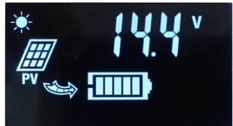
6. Floating charge voltage setting
